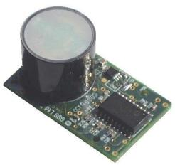
Once powered up, it will immediately start to transmit  $CO_2$  readings twice per second. This can be read directly by connecting to a microcontroller, or can be connected to a PC using a suitable serial driver chipset.
