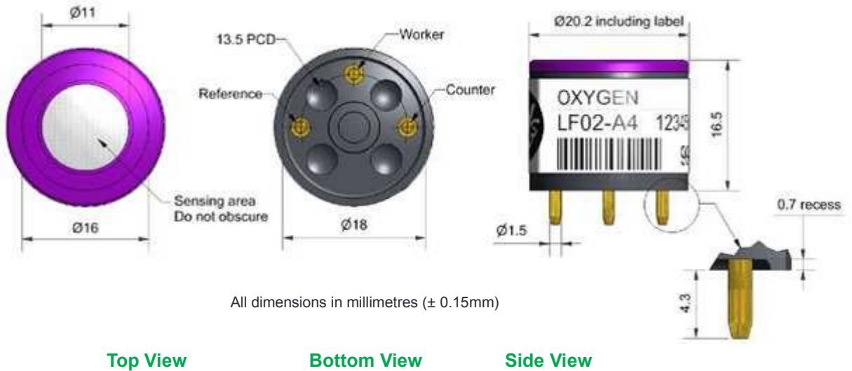
Figure 1 LFO2-A4 Schematic Diagram
