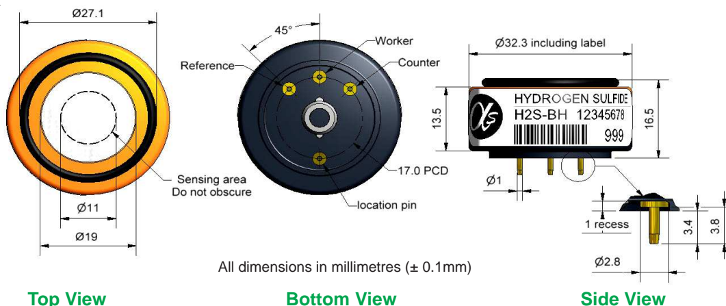
Figure 1 H2S-BH Schematic Diagram
