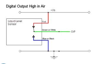
CAUTION: Take care when connecting loads. The minimum load impedance should not exceed Vs/max output current.
