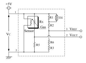
VC: Circuit voltage VOUT: Output voltage VREF: Reference voltage
